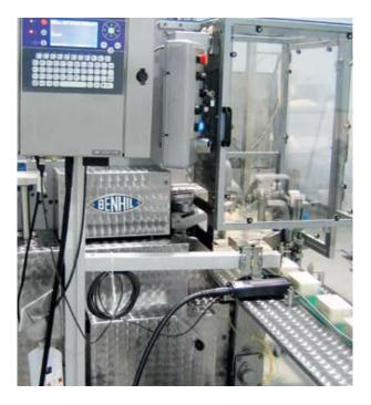
At Gower View Foods, the 9020 inkiet prints directly onto packs at speeds of up to 7,200 packs per hour.
